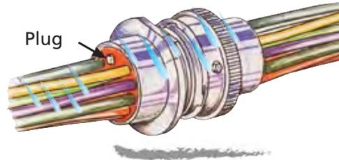
**Contact Crimp Sleeve Reducer Assembly**
