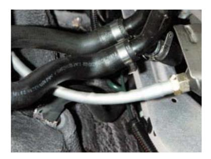
**Bentley-Harris® Textalu 1202** is an insulative fiberglass sleeving with a heavy aluminum coating designed to protect components in high temperature areas. It provides superior insulation to components that must maintain stable temperatures to assure performance efficiency.
